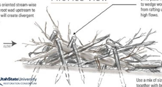
Figure 17. Typical schematics of a channel-spanning PALS. Channel spanning PALS are designed to be passable by fish at all flows. From Chapter 4 of Wheaton et al. (2019: http://lowtechpbr.restoration.usu.edu ).
