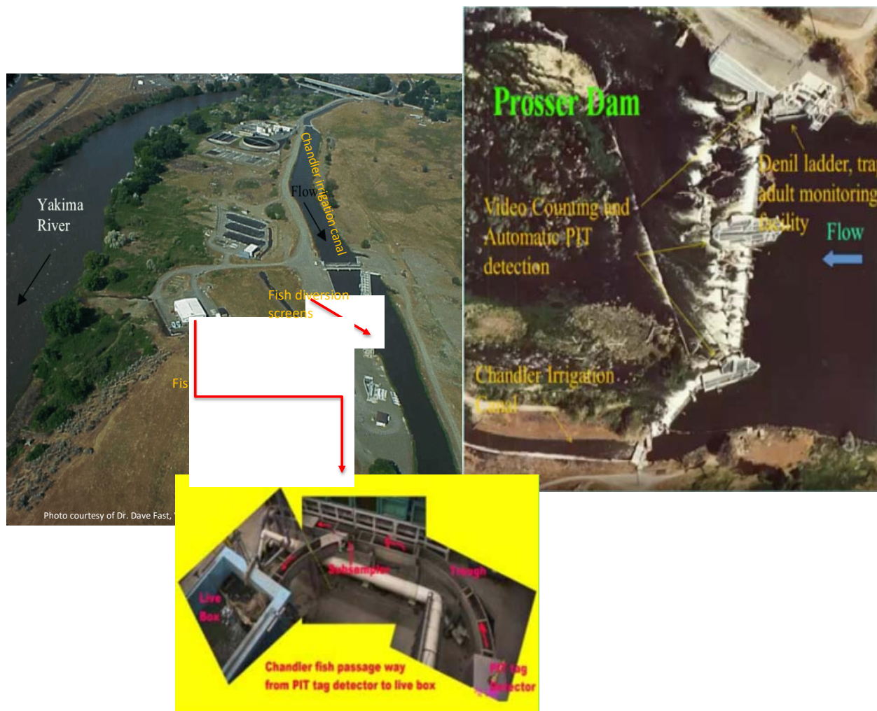
Figure 2. Composite photo depicting the Chandler canal location and the key sampling components at the Chandler Juvenile Monitoring Facility (CJMF).
