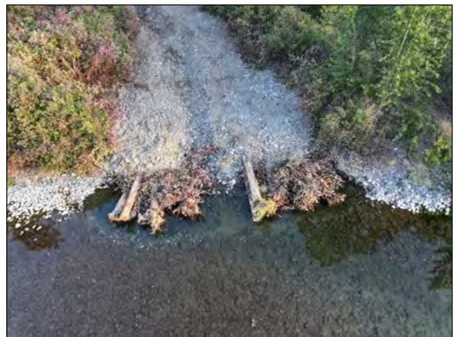
Aerial image of side-channel outlet with bank-buried large wood structures, with outlet dry at September 2025.
