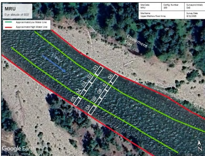
Photos above: Array configuration and installation of the PIT-tag detection system.
