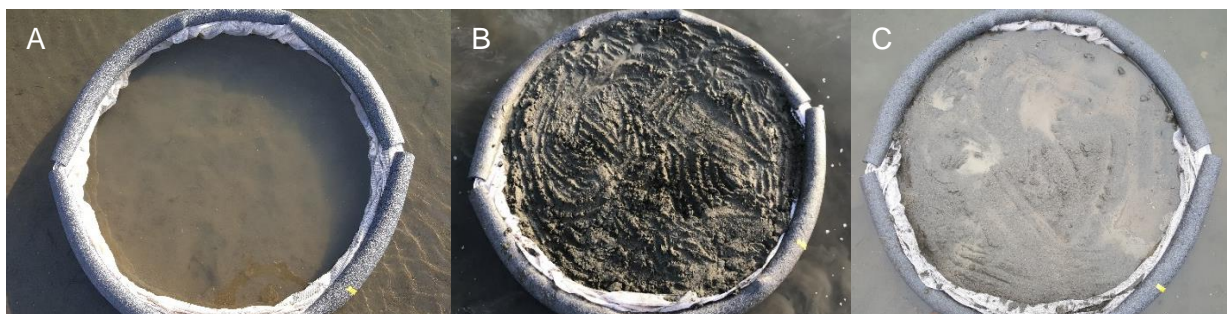
Figure A-8. Examples of the sediment levels at various points of the study: A) the starting condition prior to any sediment addition, B) after ~10 cm of fine sediment was added, C) after the top 2 cm of fine sediment was excavated down to the surrounding water level.
