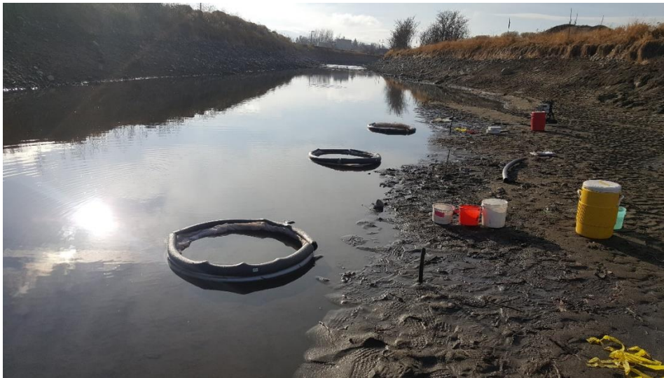
Figure A-7. Overview of the initial setup with the three enclosures on shallow fine sediment larval lamprey habitat.
