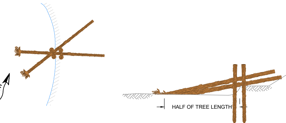
2-LOG CROSS STRUCTURE - RIGHT BANK PLAN AND SECTION VIEWS
