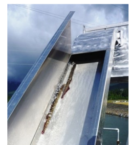
Experimental lamprey ramp design
